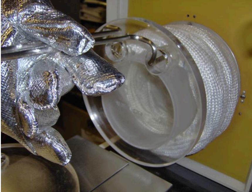
Fig. 3 Opening the door with the door support tool, notice the heat gloves are being used.
