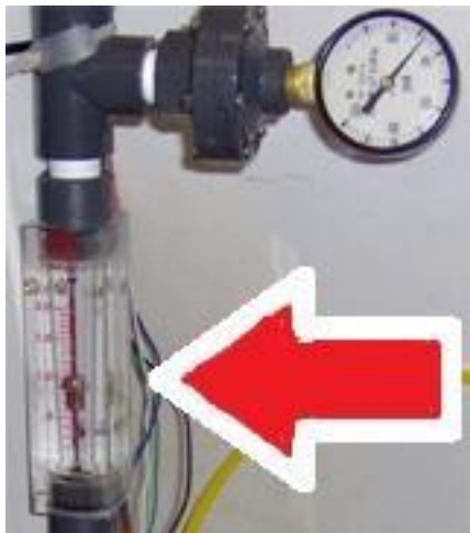
Fig. 2 Confirm the water is flowing before starting, the metal indicator should be in the middle of gauge.
