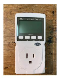
Just plug the meter into an outlet and plug the device you want to measure into the meter. Some of the values a typical Watt meter provides are Watts, Volts, Amps, kilowatt hours, Amp hours and power factor. This is a huge help when doing an energy inventory. If you let the device run for a given period of time you will get more accurate information for your inventory.
