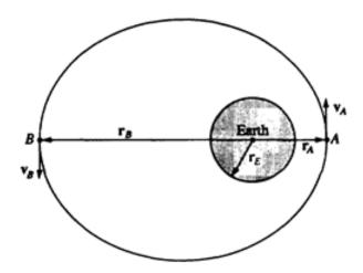
A spacecraft of mass 1,000 kilograms is in an elliptical orbit about the Earth, as shown above. At point A the spacecraft is at a distance  $r_A = 1.2 \times 10^7$  meters from the center of the Earth and its velocity, of magnitude  $v_A = 7.1 \times 10^3$  meters per second, is perpendicular to the line connecting the center of the Earth to the spacecraft. The mass and radius of the Earth are  $M_E = 6.0 \times 10^{24}$  kilograms and  $r_E = 6.4 \times 10^6$  meters, respectively.
