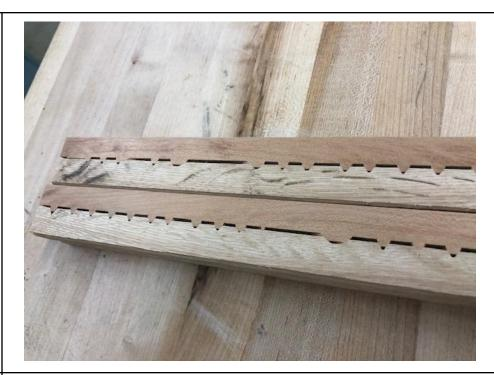
Clamp the two halves together with even pressure. Long reach clamps or cauls are needed. Do not over tighten and smash the V-carves.
