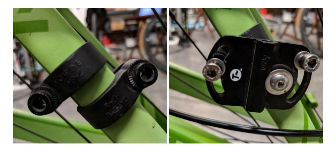
Once the clamp is installed, you can push the flag pole into it (**first image below**) and tighten the bolt head on the flange with a 3mm allen wrench. This tightens down on the pole assuring it stays in place.
