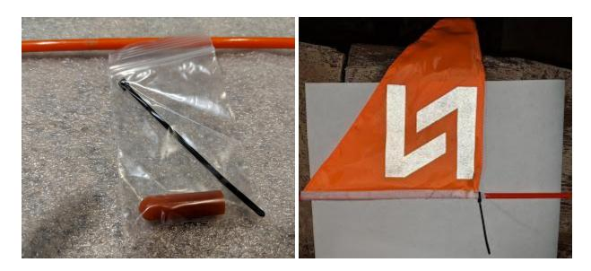
Open up the Terracycle Safety flag mount. There are instructions for installing the mount on your bicycle included. It is important to use the right sized clamps for your bike. The clamps are installed with a 4mm allen. Below are images of the mount installed with the small clamps on the seat support of the S40.
