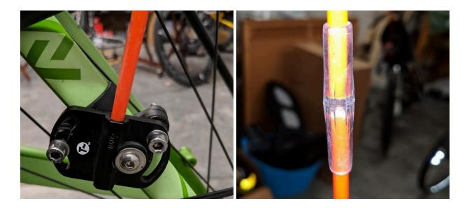
For installation on the back on the Q45 or the T50. We install the flag on the seatpost. It is possible to use only half the flag.
