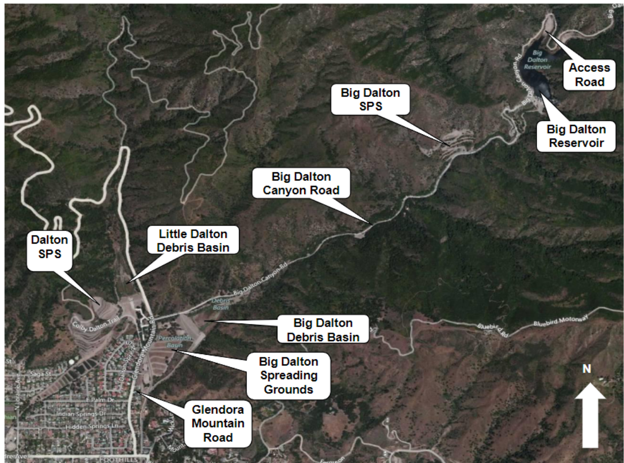
Figure 15: Water drainage in Big Dalton and Little Dalton Canyons. The Big Dalton Reservoir contains water held up by the Big Dalton Dam. Water is released into Big Dalton stream and flows to the debris basin. It can then be diverted to the spreading grounds or into the Big Dalton wash where it ends up in the San Gabriel River. The Dalton and Big Dalton SPS are sediment placement sites where sediment from the debris basins is temporarily placed before being trucked out of the area.
