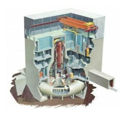
This cutaway diagram shows the central reactor vessel and thick concrete containment in a typical boiling water reactor of the same era as Fukushima
