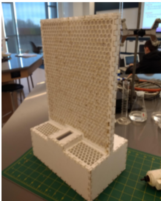
Image 4. Prototype of a coin collector for Manna Food Center made with a laser cutter.
