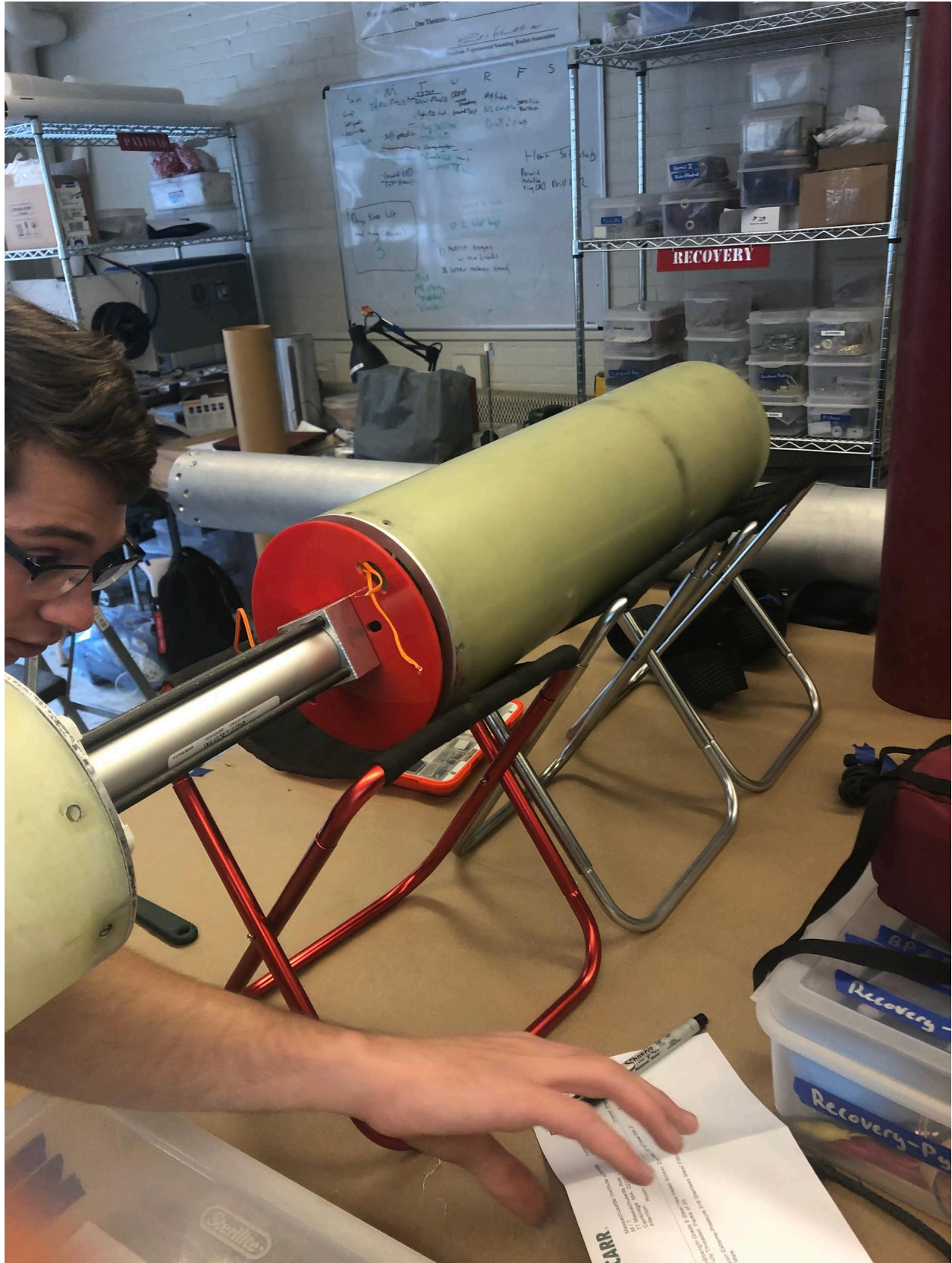
a. Attach AV tower to payload bulkhead with 6-32 bolts
