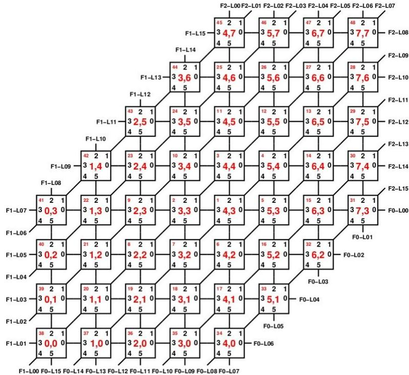
The FPGAs are connected internally to a subset of the border chips on the board as shown above; the links at the edges of the board are coded as F<fpga-id>-L<fpga-link-id>, so F1-L04 is FPGA 1, FPGA link id 4.
