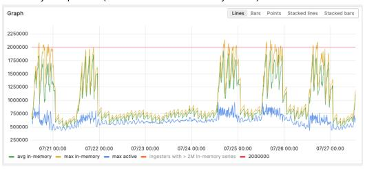
When early compaction triggers, in-memory series in that ingester drop to active series:
