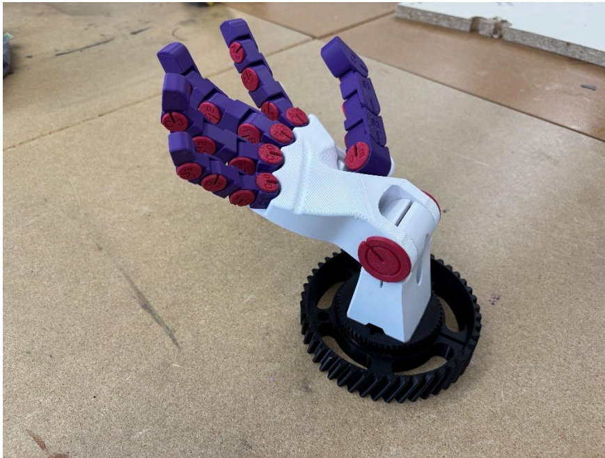
3-D printed mechanical hand created by student and Collaboratory volunteer, (Pin-Yu) Amy Lin.
