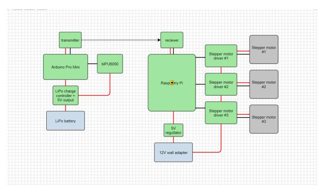
Red is Power Black is Data Dotted Line is wireless transmission over radio
