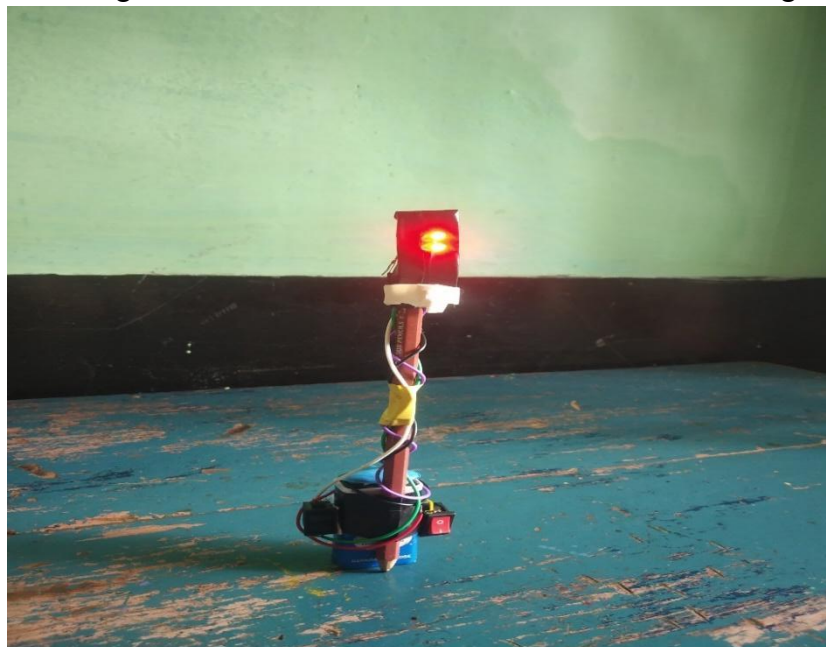
Figure 20. Traffic indications model with red and green led lights
