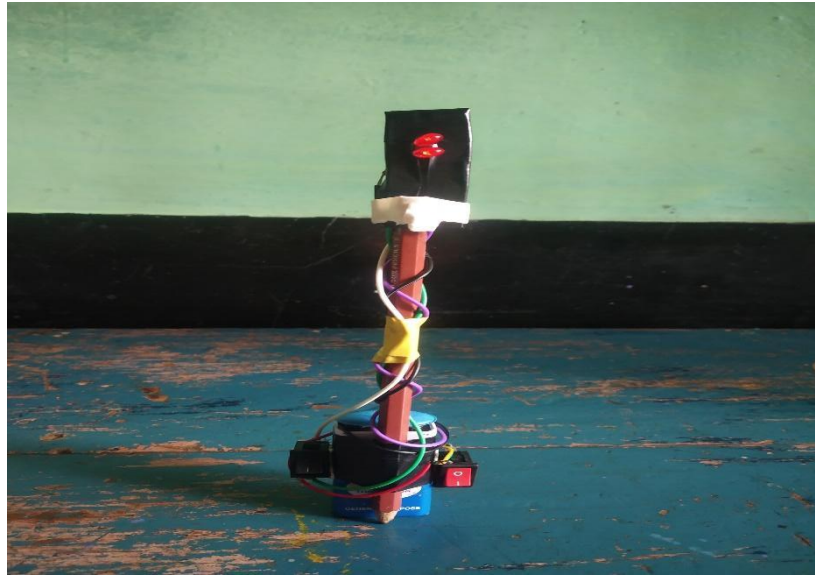
Figure 20. Traffic indications model with red and green led lights
