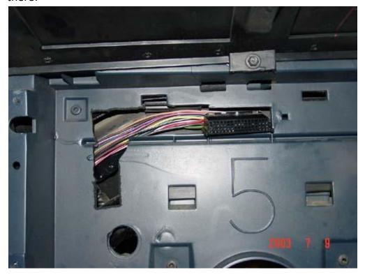
I decided to place my DRAC behind my radio.....b/c it fit and was less of pain than running wires to the glovebox....Gotta clip the DRAC like the blue is shaded in the previous pic of it. I got some 18 gauge wire and fed it through the cluster opening, and fished it out of the radio hole with a coathanger. Did this 8 times. Wire went in the left green spot, came out the right green spot:
