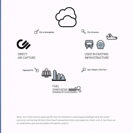
Above: Air-to-Fuels involves capturing CO<sub>2</sub> from the atmosphere, producing green hydrogen with low-carbon electricity, and reacting the two to form liquid transportation fuels such as gasoline, diesel, or Jet-A. Such fuels can be closed carbon cycle and can displace the need for crude oil.
