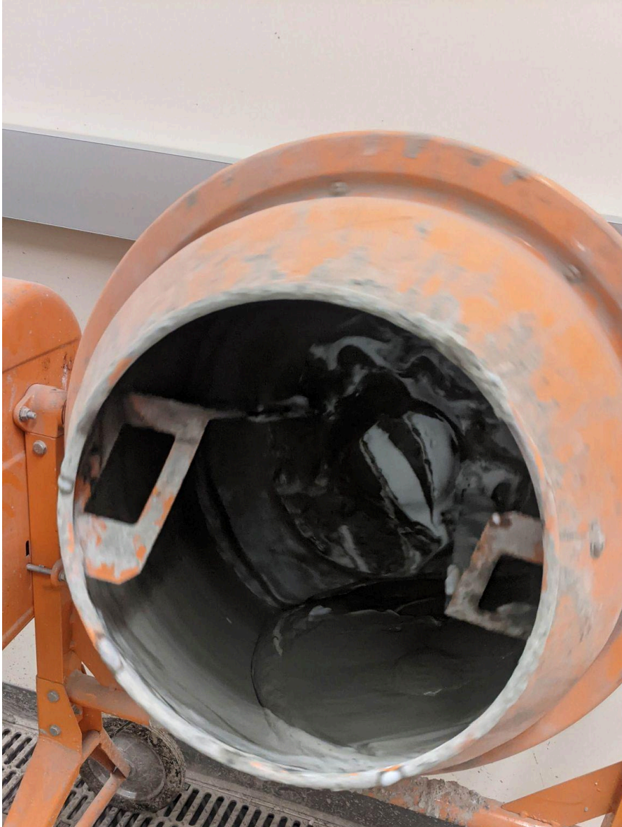
Below left to right (Aircrete created in mixer, 2 collapsed aircrete using auger)
