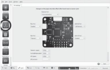
If your transmitter and receiver have already been setup with the flight controller, this page can be used to test the transmitter controls and switches. The flight battery
