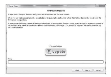
When the update is completed, click on the Next button to open the Board Identification page. The detected board should be "CopterControl 3D". Cancel the wizard to return to the Welcome screen.
