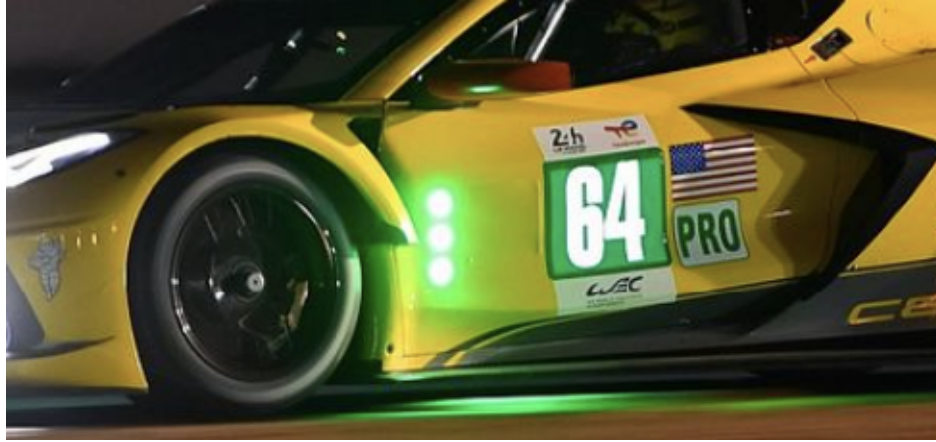
fig. 1.3.4: an example of position indicator light
