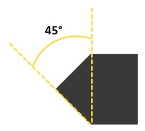
Overhanging features at angles more than 45° from vertical may require support, though some printers/materials can go up to 60°. Horizontal holes and channels smaller than ¾" diameter usually do not need support material, but shrinkage of horizontal holes and internal cavities tends to be more significant in the direction perpendicular to the layers than in other directions.
