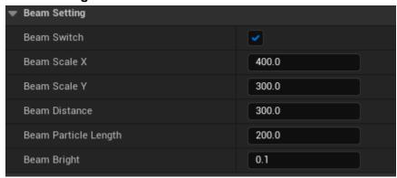
Beam Switch: Switch that can turn the beam effect on and off
