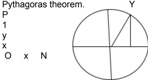
The figure above shows a unit circle.  $\triangle OPN$  is a right angled with  $OP = 1$ ,  $ON = x$  and  $PN = y$ ,  $\angle PON = \theta$ . From the definition of trigonometric ratios.
