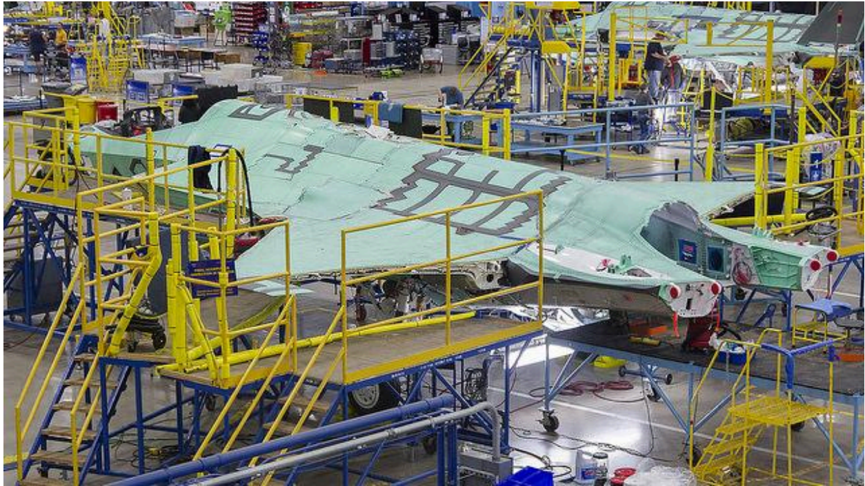
Norwegian Ministry of Defence via Flickr Close up of the first Norwegian F-35 production line
