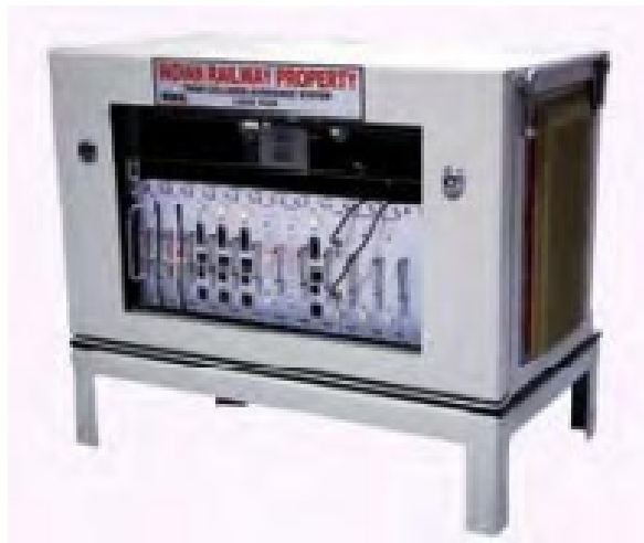
Loco TCAS unit
