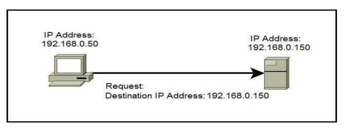
In the picture above you can see that the host wants to communicate with the server. It uses the (unicast) IP address of the server (192.168.0.150) to do so
