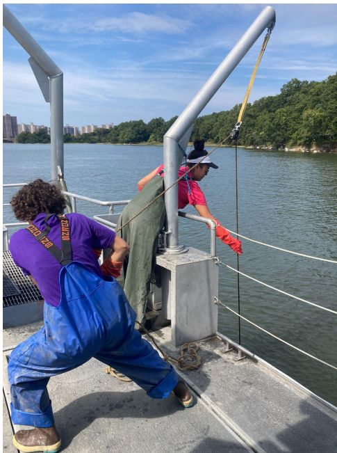
BOP scientists use a tool called a ponar grab to pull up a small sample of sediment from the seafloor.
