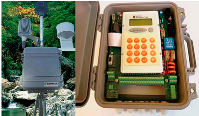
Figure 0: Weather station ( Geonica Meteodata 2008CP ) and sensors.
