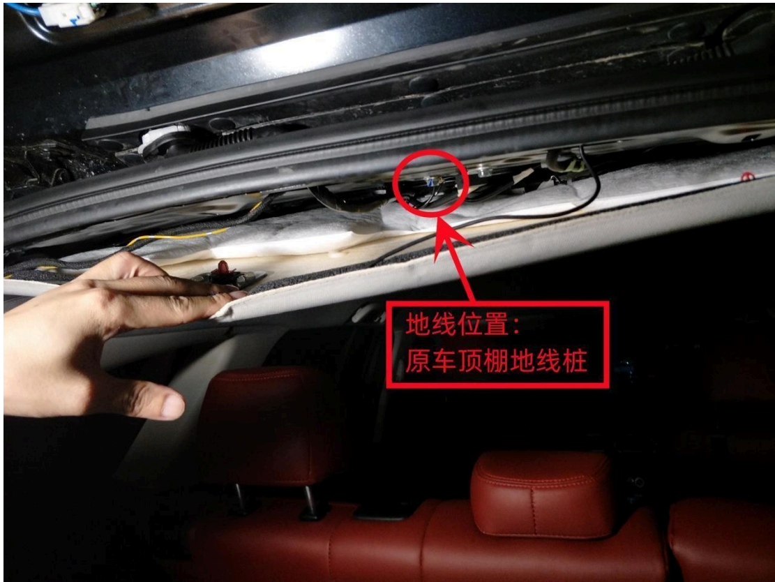
Ground wire location: Original vehicle roof ground wire terminal
