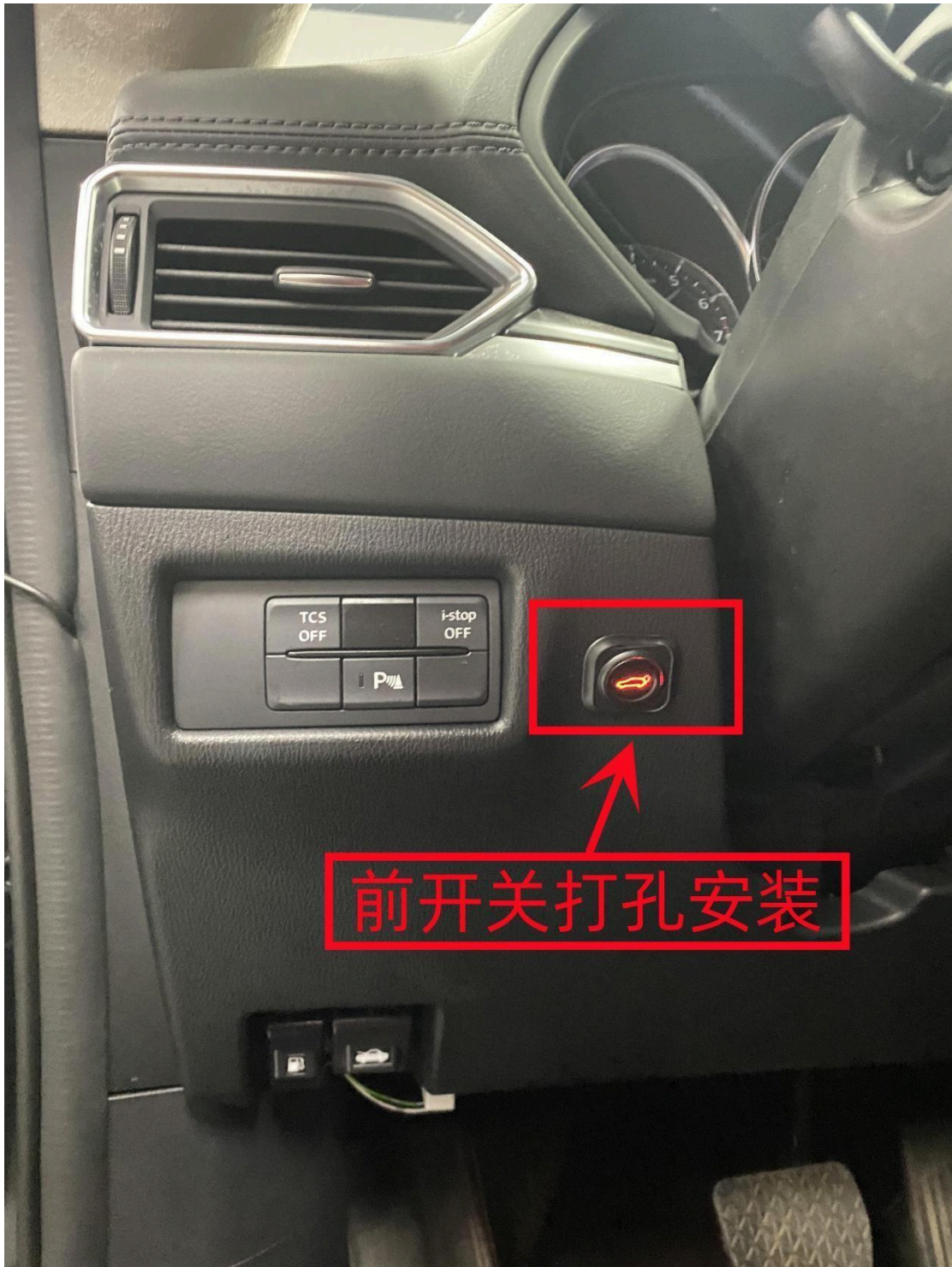
Drill holes and install the switch.
