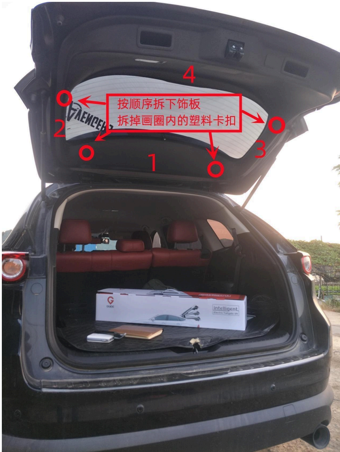
Remove the trim panels in the correct order. Remove the plastic clips within the red circles.
