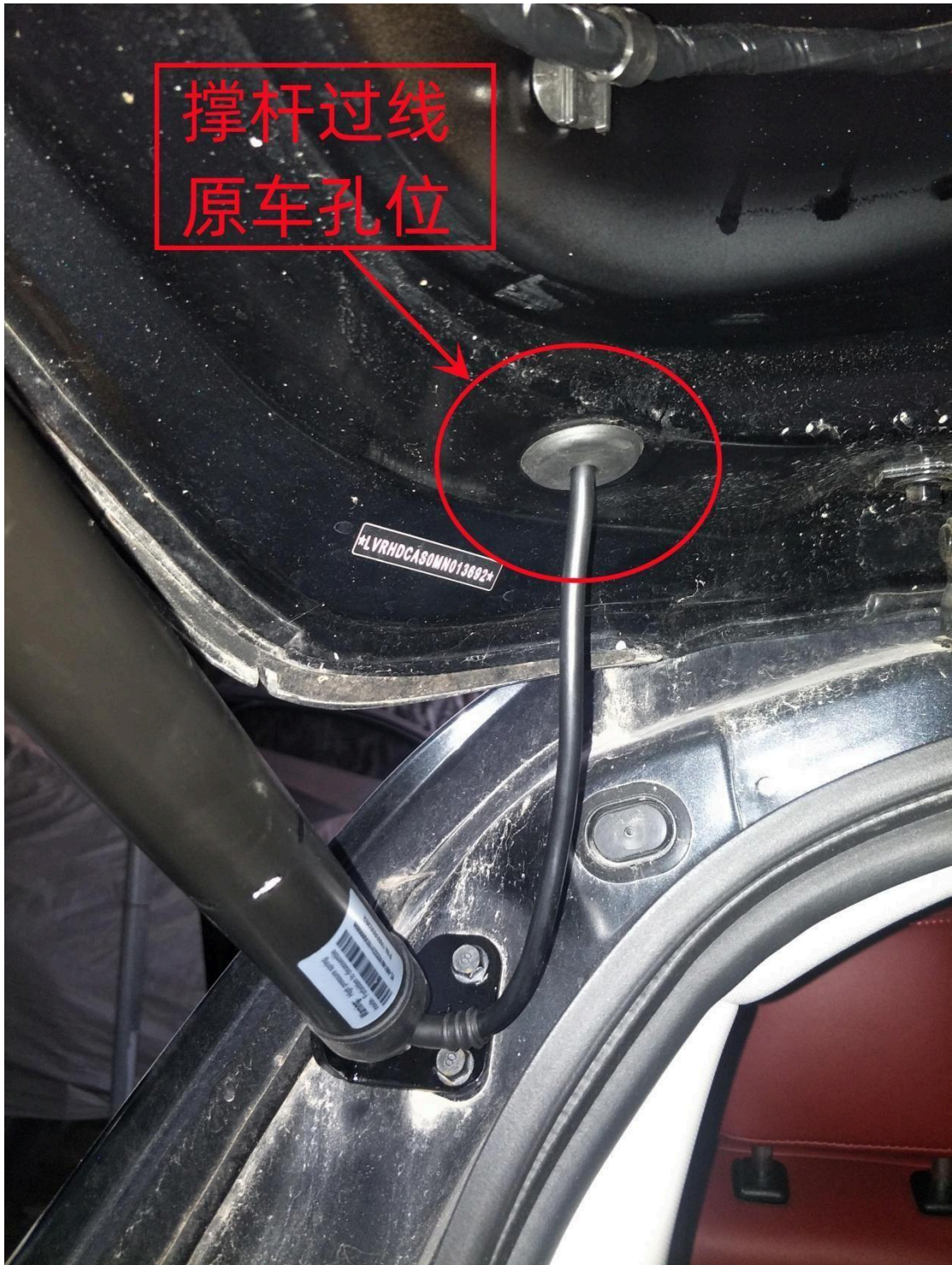
Strut mounting points utilize the original vehicle's mounting holes.
