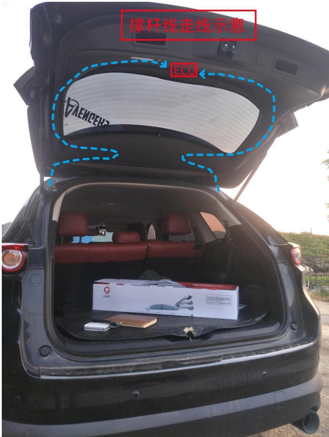
Diagram showing the routing of the struts wires.
