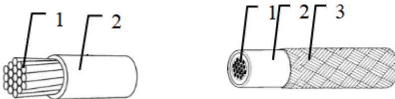
1—Conductor; 2—Insulation; 3—Shield;
