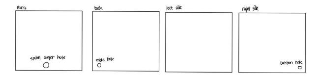
**9.** Cut and drill the holes in PVC pipe and container. You need to cut the PVC pipe at an angle. You will also have to use a drill press to drill a hole in the dog food container and the PVC pipe (see the picture below).
