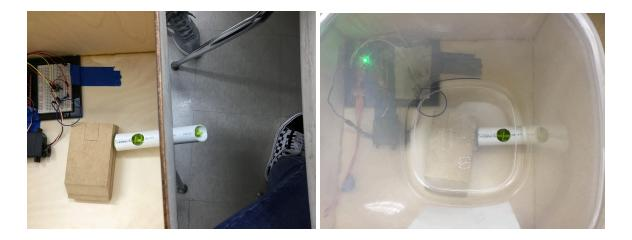
10. **Assemble the dog feeder.** First, insert the PVC pipe into the larger hole. Above the PVC pipe should sit the container (the holes aligned) Then, glue your arduino inside along with your servo and cable. Run the cable through the smaller hole. Your servo, along with the attached spiral auger, should slide into the PVC pipe. If your servo cannot support itself, complete step 11. (See the image below for a visual.)
