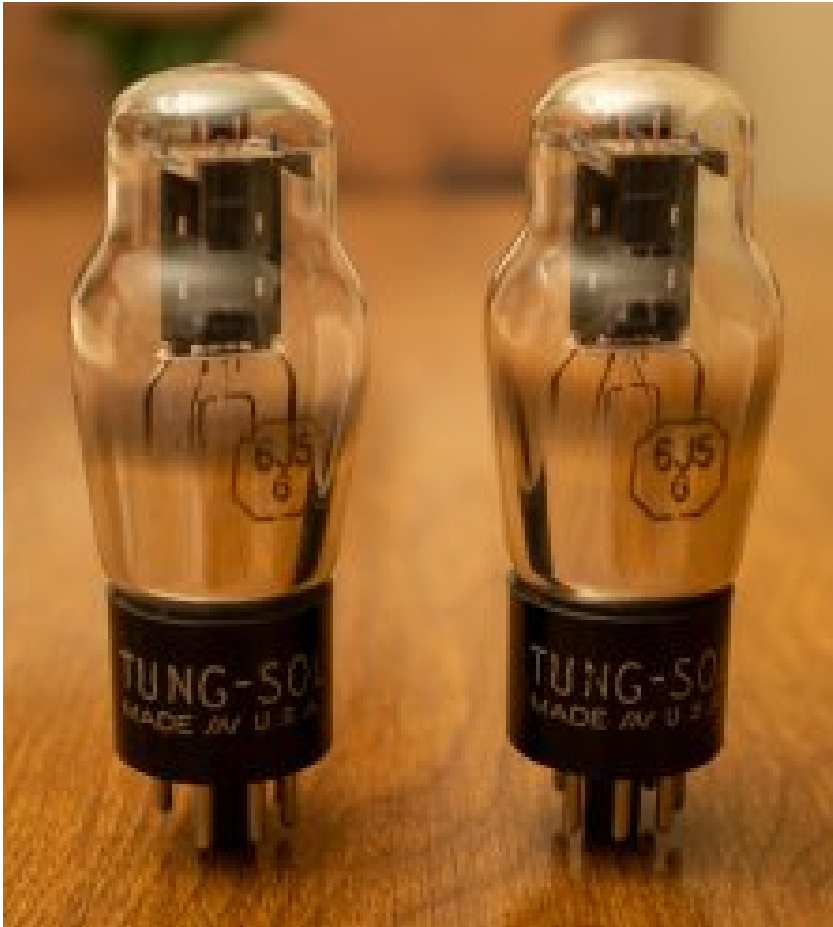
(photo: L0rdGwyn) -ladder plate (same construction as Tung Sol black glass round plate 6SN7GT) -foil getter
