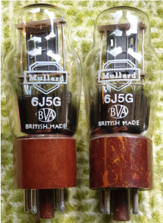
(photo: chrisdrop) -brown base (uncommon) -serrated top mica -thin rectangular bottom mica -double support rods -can be labelled CV1932 Bottom rectangular getter -Tungsram factory
