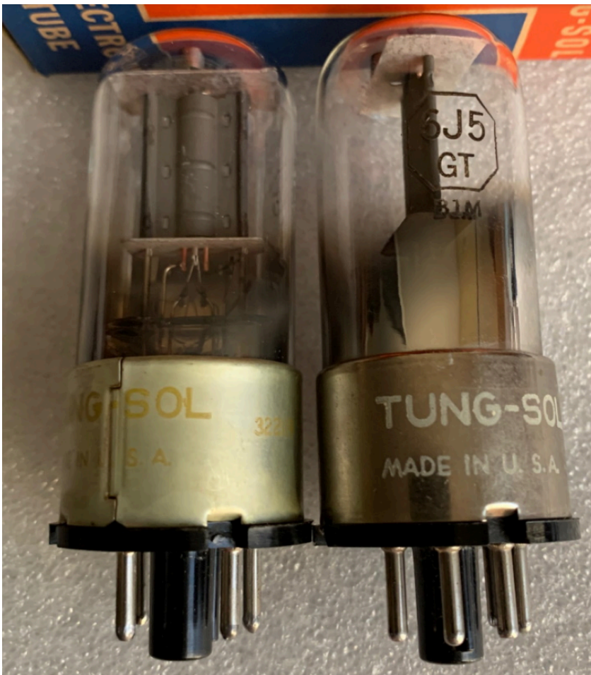
(photo:bcowen) -Tung Sol round plate -ladder style type plate (right) = likely rebrands of Sylvania
