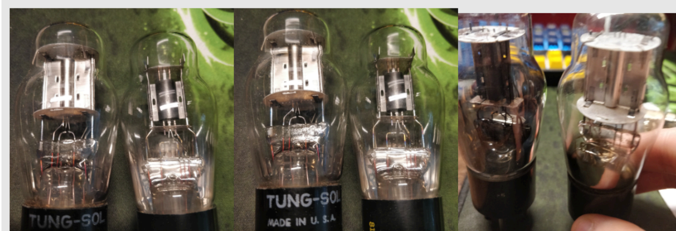
Last of the 3 images is the Tung Sol 6L5 compared to an RCA 76. Note the top mica similarities. I don't know of another brand to do top micas like this.
