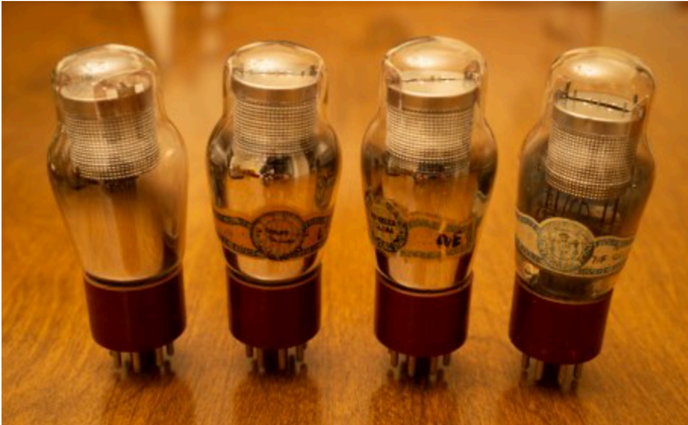
(photo: L0rdGwyn) -brown (or black?) base -shorter bottle -mesh shields -wire spacers replaced by mica
