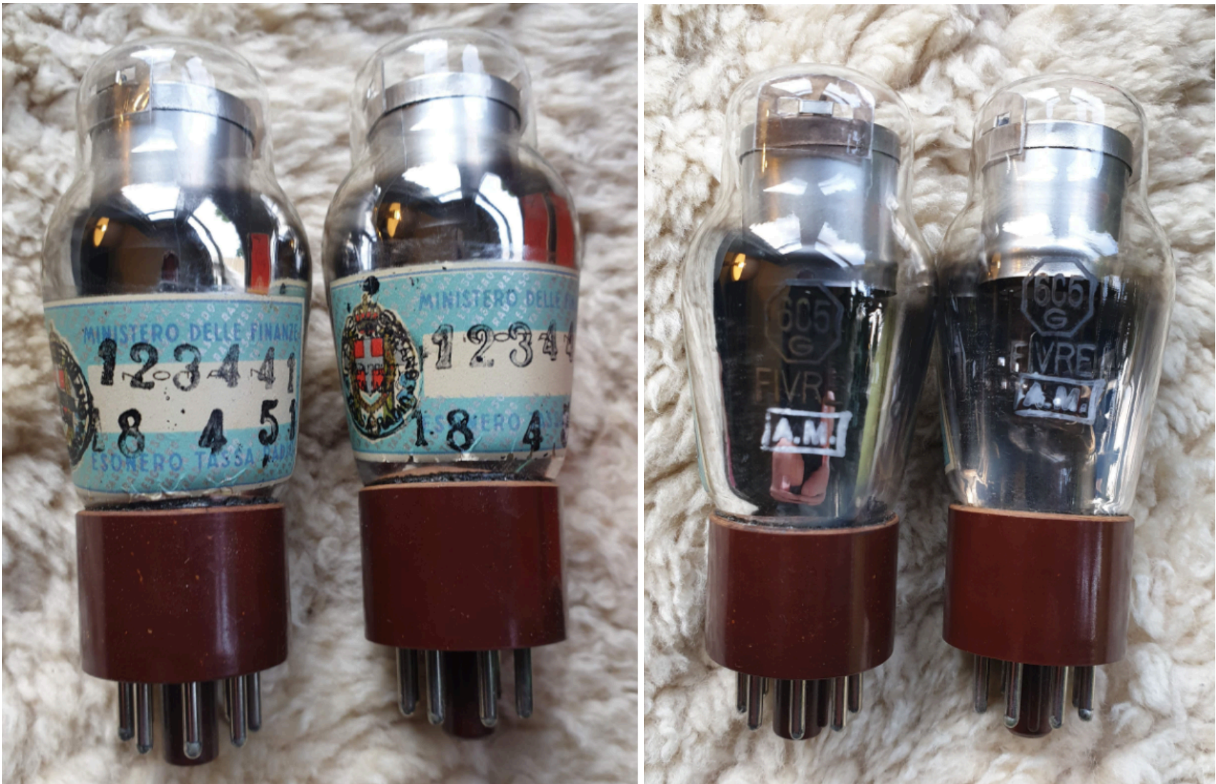
(photos: chrisdrop) -solid instead of mesh shields
