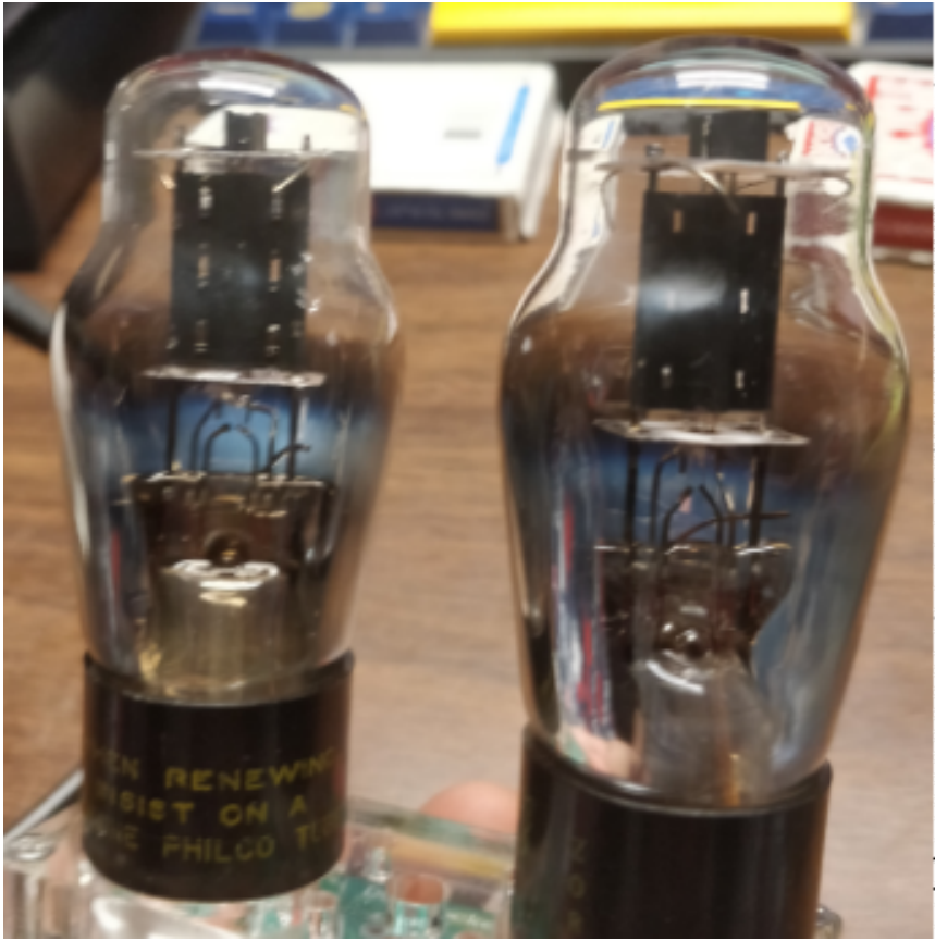
(photo: RoyGB) -3 hole plate similar to Sylvania 6J5GT -U shaped top heater shield
