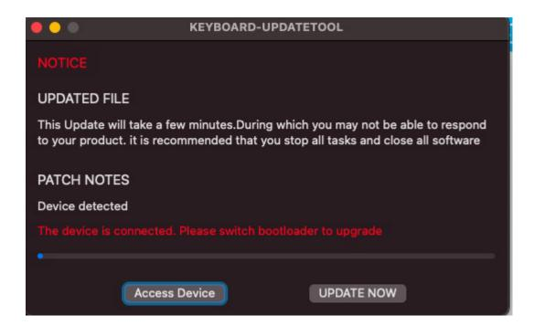
3. When the prompt box displays "Bootloader device inserted detected, please upgrade", click the button on the right "UPDATE NOW" (note: only need to click once):
