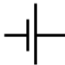
Figure 2.8. Symbol for battery. The short end is the negative terminal and the long end is the positive terminal.
