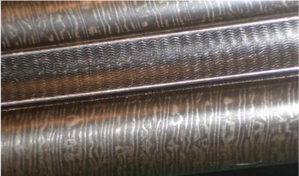
A Twist pattern refinished in “black & white” by Paul Stevens with “mushrooming”. An “end on” rod in the middle.
