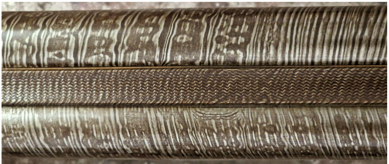
A Twist pattern refinished in “black & white” by Paul Stevens with “mushrooming”. An “end on” rod in the middle.
