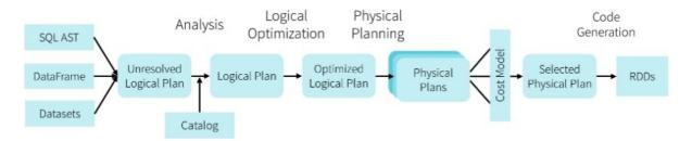
Spark positions the catalog resolution at the level of the Logical Plan. It has an extra state for the query that is not present in DataFusion: the **Unresolved Logical Plan**.
