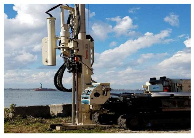
pushed into the target depth then pushed more into the aquifer. An aquifer is a porous rock that lets water pass through it.
