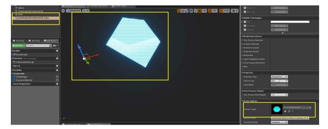
First, place an object you want to capture on BP\_SceneCapture (refer to the existing position value carefully) and then create a camera component or use an existing component. Next, please adjust the angle and position of it so that it can capture the object well. Next, set the RenderTarget to contain the captured image.
