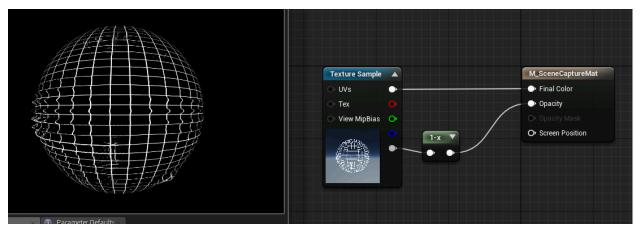
Finally, the Render Target containing the captured information is called from the material and set. You can now use this material as a UMG in the image widget.
