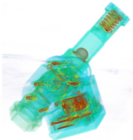
Example 3D rendering of the object reconstructed from the above radiographs
