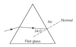
**8.** Calculate the angle of refraction (in degrees) of the light ray as it enters the air from the flint glass prism.
