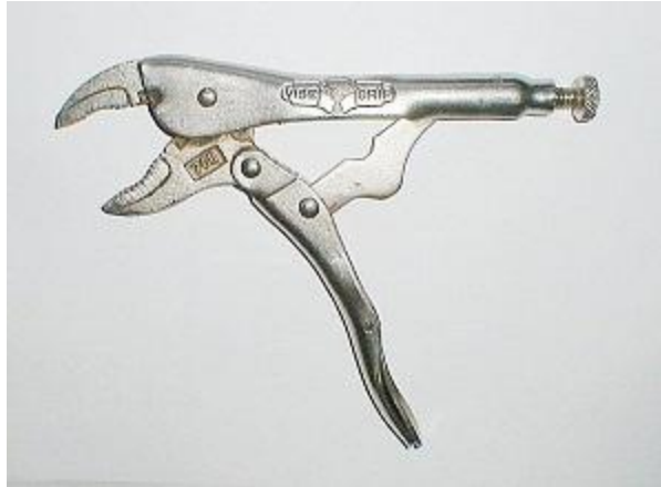
This pair of locking pliers contains non-two force members and has parts that can move relative to one another (it is not rigid). Therefore this is a machine
