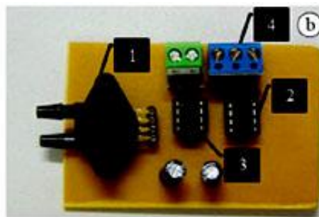
Figure 2. (a) Electronic circuit used to capture the signal with the sensor MPX10DP. (b) Circuit board (PCB): (1) - Sensor MPX10DP. (2) - Operational Amplifier TL072CN. (3) - Instrumentation Amplifier INA118P. (4) - Connectors to power supply.
