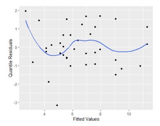
In looking at this plot, we can see that the line is extremely bumpy. While it is around 0, I would not consider the line flat. Therefore, I would say it does not pass the test. Additionally, there seems to be an outlier below -2.5 for Quantile Residuals that is skewing the data
