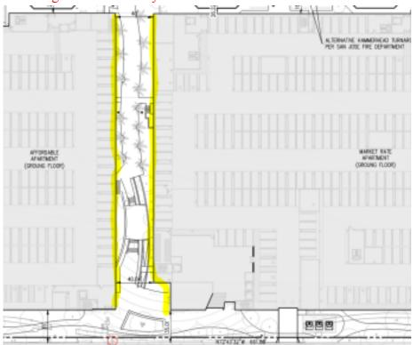
• Where a fire hydrant is located on a fire apparatus access road, the minimum road width shall be 26 feet, exclusive of shoulders.
