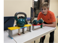
The well constructed bridge holds 15 pounds easily while the poorly constructed bridge bends while holding only 8 pounds
