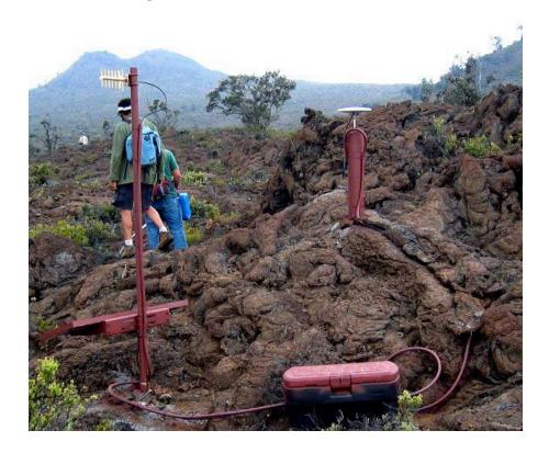
Figure 2. A GPS unit installed at Hualalai volcano, Hawaii. The dish-shaped antenna on the right is the GPS receiver. The antenna on the left is for communication with a base station. [from USGS at: http://hvo.wr.usgs.gov/volcanowatch/view.php?id=173]
