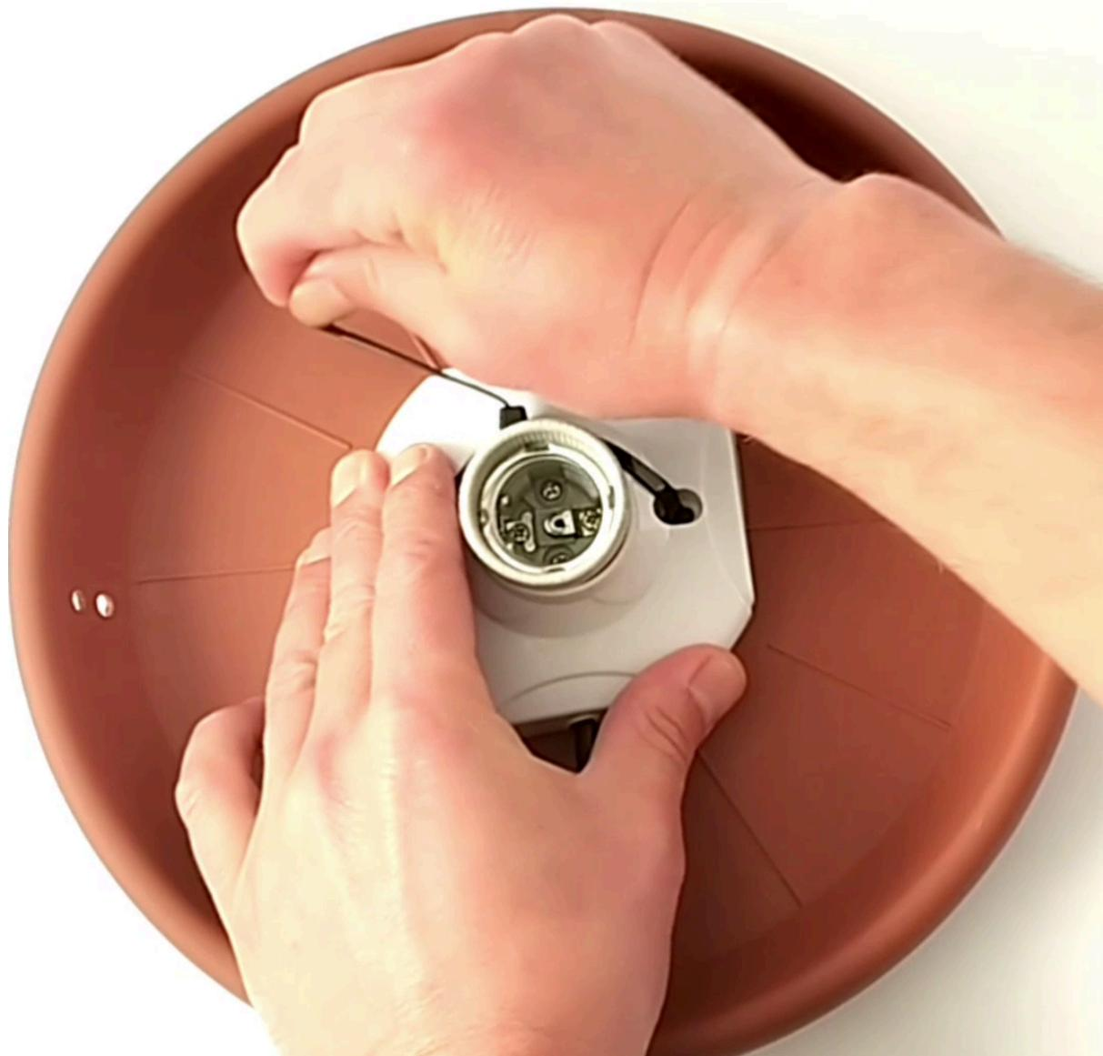
Step 11: Use the 100mm cable tie to secure the power cable to the inside of the plastic saucer for strain relief. This way, if anyone pulls from the cable to move the heater, they will be pulling from the cable tie and not from the bulb holder terminals.
