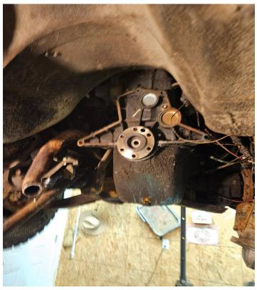
After i pulled the transmission and clutch i soaked the flywheel bolts in kroil and pulled that, we will be replacing the stock flywheel with one off of a 4.0, i had a used one in good shape but aftermarket replacements are available.
