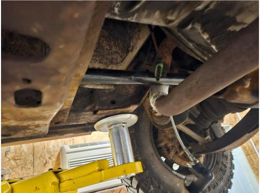
Welded some bracing in to maintain strength of the crossmember then went ahead and welded my crossover pipe back in.
