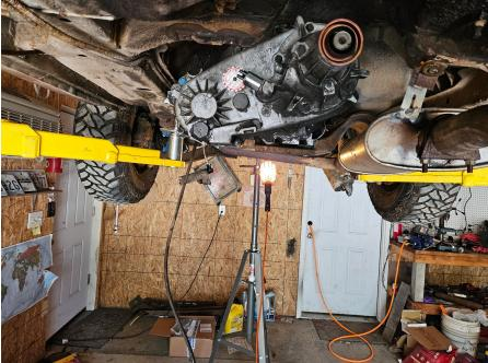
Make sure to use the cherokee spacer plate when you install the transmission, i didn't and had to take the trans back out as the bottom of the bell housing is shaped just different enough for the eagle one not to work.
