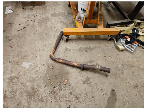
Step number one was removing the old transmission, instead of fighting the locked up rusty exhaust bolts i just cut the crossover pipe off. I found the easiest way to get the old trans out was to unbolt it from the bell housing and pull them separately.
