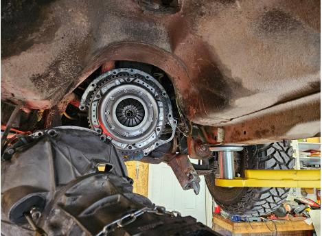
Once the new flywheel and clutch were mounted up it was time to slot the new trans into place, it was a bit of a squeeze but once you get the input into the clutch you have plenty of room to wiggle it home.
