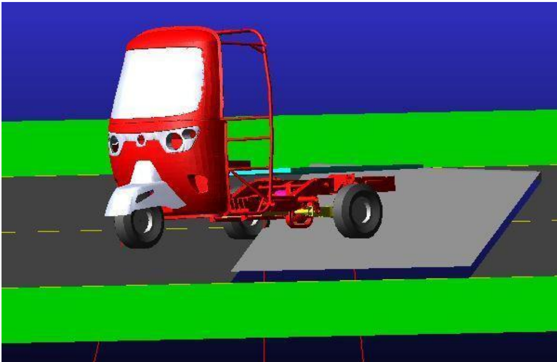
Simulation on MSC Adams View for extracting Load data
