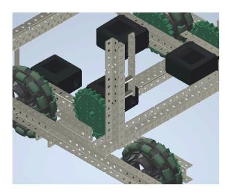
11. Attach an 8-hole half-channel to the vertical bar using two standoffs on the sixth and eighth hole.
