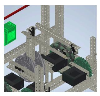
29. Attach pillow blocks to each of the screws extruding from the half-channel. Add two standoffs to each pillow block.
