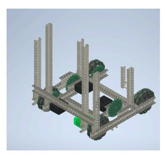
13. Next, we build the lift towers that hold up the lift. Two C-channels that are 22 holes long are added to the ends of the base. These C-channels should be oriented in a way that they are facing outside. Two other C-channels that are 35 holes long will be placed on the inside of the base. All four C-channels are going to have one of their sides attached to the horizontal crossbar. This will contribute to the lift's sturdiness.
