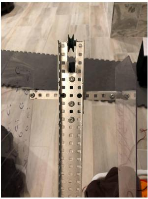
36. Attach two polycarbonate panels on each side of the tray using a perpendicular screw joint. To make the screw joint, use one screw that goes through a collar, then have a screw extruding from the horizontal hole of the collar. Make sure to secure the screw initially with a nut.
