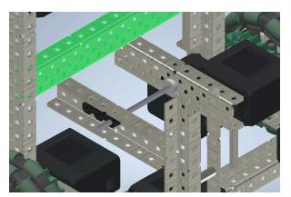
23. Attach an axle to the motor and add a bearing to the C-channel on the left.
