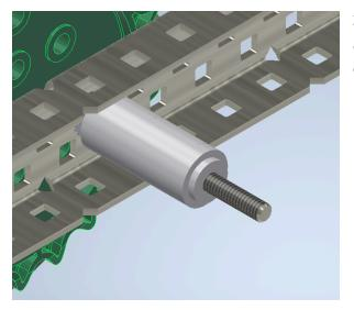
31. On the screw that has just been attached, add one inch of spacing and a one sixteenth spacer.
