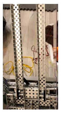
35. For our second level of the tray. This is made up of two C-channels that are 35 holes long. To attach this level with the first level, use two bearings and attach two standoffs on each side to a 3 hole side C-channel.
