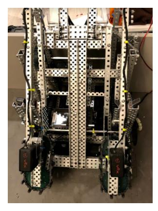
34. Attach two C-channels that are 35 holes long to the 3-hole-wide C-channel. These two C-channels should be attached to each other and the crossbar on top of the lift towers.
