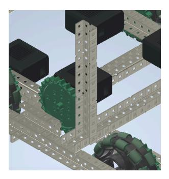
10. In order to prepare for building the actual lifts, we will be building vertical bars. These are made from C-channels that were fourteen holes long. These vertical bars will be used to align the lift.
