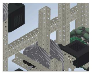
24. Put a high-strength gear, a C-channel, then another high-strength gear on the axle attached to the motor.
