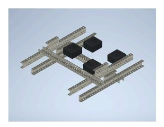
5. Attach four 200 RPM motors to the base. Two of the motors should be attached to the two inner initial C-channels, while the other two should be attached to the small six-hole-long C-channels.
