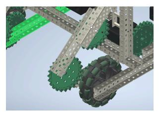
19. Attach a C-channel to the lift arm. Then, on the bottom of the C-channel, attach one sprocket via screw joint near the bottom of the C-channel. Attach a motor on the upper part of the C-channel (not shown in image) and attach another sprocket to the motor using an axle. Mirror the rollers on the other lift arm.
