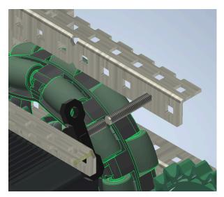
28. Put a screw through each half-channel one hole away from the edge.
