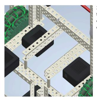
21. Attach a C-channel that is 10 holes long to each standoff. These C-channels will be oriented with the flat parts facing each other.
