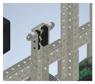
26. Put two screws through the top hole of the bearings that has a Keps nut, then a collar.
