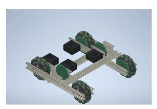
7. On the same axle as the outer sprockets (not the middle one), attach a 4-inch omni wheel to each axle. Make sure to link all the sprockets together by connecting chain links on the sprockets (not shown in image)
