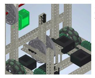
25. Attach two bearings, each on either side of the C-channel that is attached to the gears.
