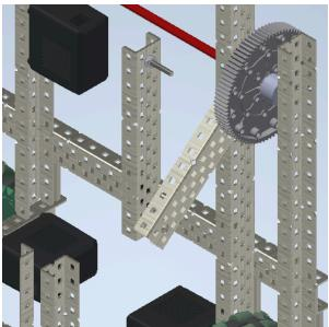
16. We need two C-channels that are each 13 holes long. These C-channels should have the flat side facing the gear so that they take up less space when they are attached to the wheel.
