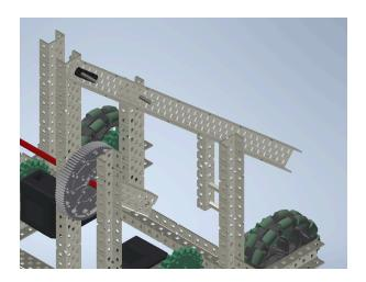
17. Attach a C-channel to the inner vertical bar via screw joint and attach it to the medium-sized C-channel extruding from the C-channel that is attached to the high-strength gear
