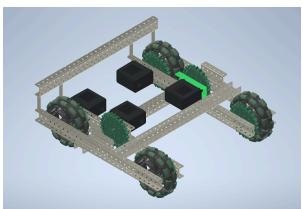
9. Add a C-channel that is attached atop the four standoffs in the back of the base.
