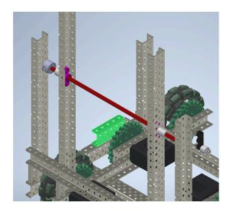
14. Run a high-strength axle through the four vertical bars. Also attach high-strength collars and high-strength bearings where needed. We will need a high strength axle in order to give the maximum support to the lift.
