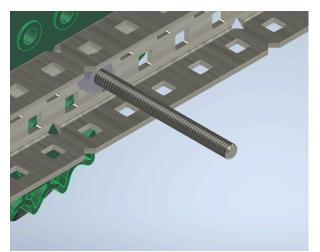
30. Attach a 1.5 inch screw on the inner C-channel. Secure it with a Keps nut.
