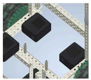
20. In order to build the angler, we first need two standoffs that are each 1.5 inches. These will use a midget to connect to the lower crossbar of the base. It is important that they are screwed on tight because they will be holding up the angler, which deal with a lot of weight that comes from the cubes.
