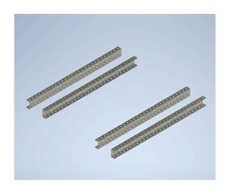
1. We start off building the base with four C-channels that are twenty-eight holes. Twenty-eight holed C-channels are necessary because we need our base to be relatively small in order to move around the field without being hindered by the vast amount of cubes that are on the field.
