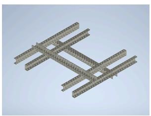
3. Similar to the crossbar C-channel attached below the base, there is also another C-channel of the same length that acts as a crossbar attached above the base.
