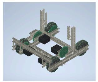
12. Mirror the vertical bar and half-channel on the other side of the base.
