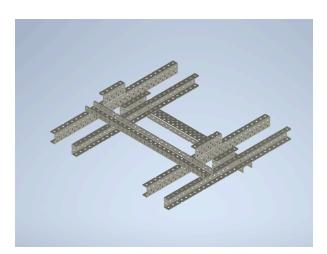
4. Obtain four C-channels that are six holes long. These should be placed in the same orientation as the C-channels that they are attached to. These C-channels are here in order to hold up the motors.
