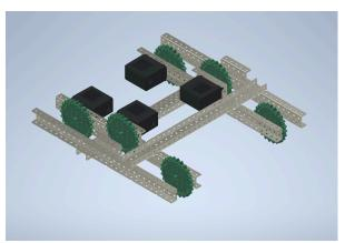
6. Attach two sprockets to the motors on each side using an axle. At the front, attach one sprocket on each side to the inner C-channels also using an axle. Make sure to apply bearings to stabilize the rotation of the axle.
