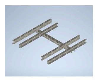
2. After orienting the four C-channels as shown on the left, we add another C-channel that is attached to all four C-channels. The purpose of this C-channel is to connect both sides of the base.
