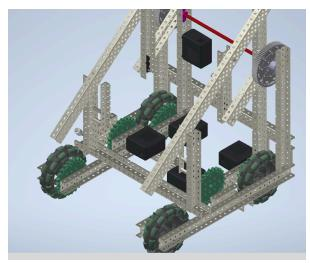
18. Mirror the high-strength gear and various crossbars on the other side of the robot.
