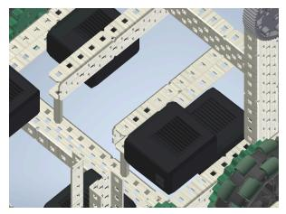
22. Attach a motor to the C-channel on the right.
