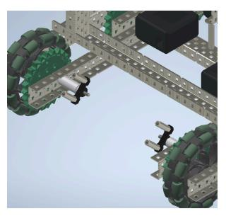
32. Mirror the screw on the other side of the base. Attach a pillow block to each of the screws. Attach two standoffs to each pillow block.
