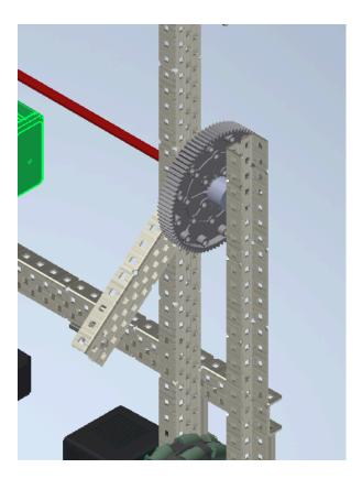
15. Attach a high-strength gear to the high-strength axle. Screw a C-channel onto the high-strength gear.
