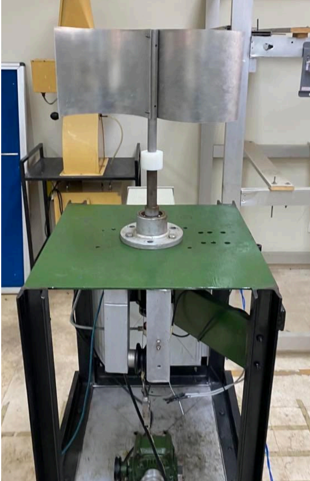
Figure 3-2: Savinous turbine with traditional blade
