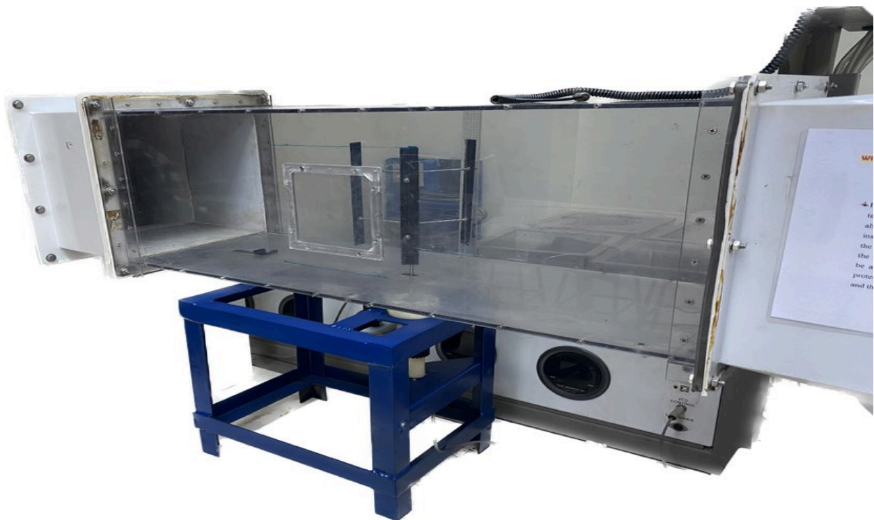
Figure 4-1: Darrieus turbine in the wind tunnel
